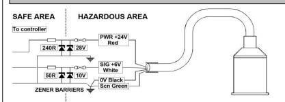
**Ex mb version:** This model must be supplied from apparatus that provides protection from prospective short circuits > 1500A.
