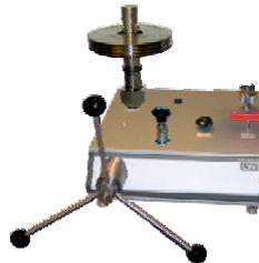
High-pressure Deadweight Tester/Pressure Balance CPB5000-HP
