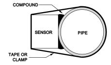
Over time temporary coupling compounds (e.g. Petroleum Gel) may gradually sag away from the sensor resulting in reduced signal strength and finally complete loss of signal. Warm temperatures, moisture and vibration will accelerate this process. Dow Corning Silicone Compound #4 as supplied with the DFM 5.1 (and available from Greyline Instruments) is recommended for semi-permanent installations.
