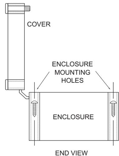
Note: This non-metallic enclosure does not automatically provide grounding between conduit connections. Grounding must be provided as part of the installation. Ground in accordance with the requirements of the National Electrical Code. System grounding is provided by connecting grounding wires from all conduit entries to the steel mounting plate or another point which provides continuity.
