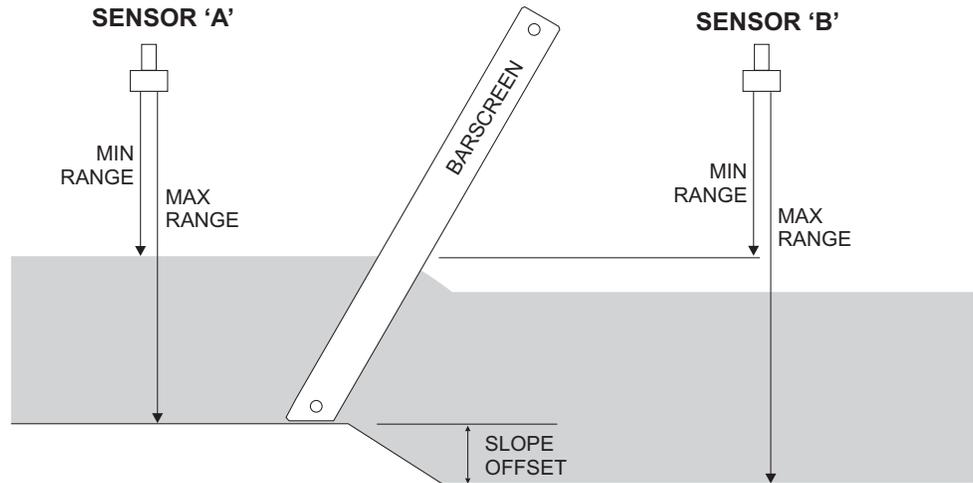
**Slope Offst** Appears when calibrating Sensor B. Enter a slope offset value to compensate for a sloped channel floor. Offset will be a positive value when Sensor B channel floor is lower than Sensor A channel floor.
