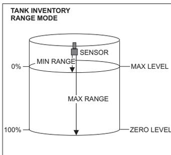
2. Check the maximum range with the sensor installed:
