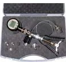
The Digital Test Pressure Gauges **LR-Cal LDM 70-K50** are available as complete pressure calibration kits (case, with calibration testpump **LR-Cal LPP 40**, **LR-Cal LPP 60** or **LR-Cal LPP 700**).
