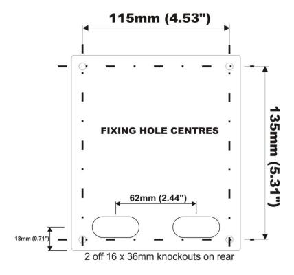
The *Flow Monitor* should be mounted by drilling four holes suitable for size 8 screws (length and type to suit your application) And fix all four screws by removing the top cover to access the pre-moulded mounting holes which are located in the base of the enclosure under the lid retaining screws.
