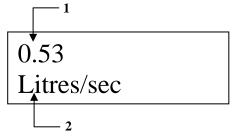
2) Auxiliary Display, scrolling 12-digit alpha numeric display Run Mode: displays units, totaliser or status messages on communications, detail of Hot Key function selected. Program Mode: displays Menu and Sub Menu headings, parameter details and options.
