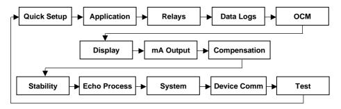
As you press the cursor keys to scroll left and right between these, you can press ENTER at any time, to select the desired menu heading, and take you to the sub-menu.
