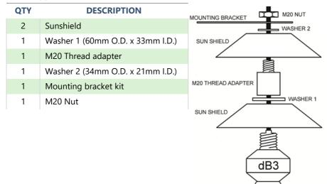
The upper sun shield is held in place by the mounting bracket and the M20 nut. The bracket can be fixed using the supplied 'U' bolts.
