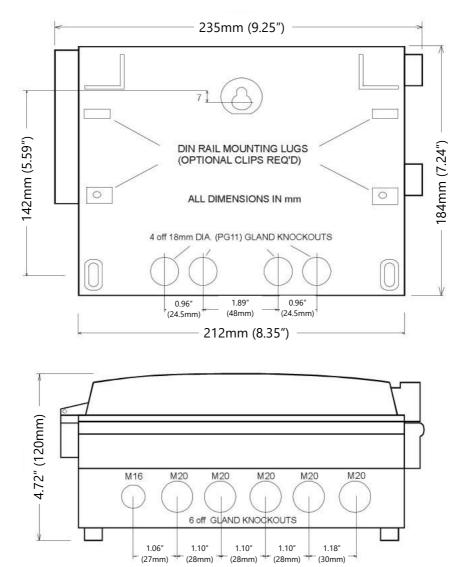
The full dimensions of the enclosure are as shown below:
