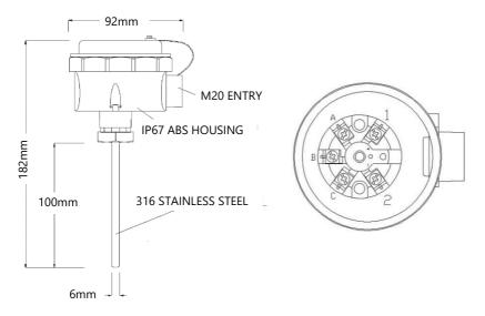
The Temperature sensor connections are as follows:
