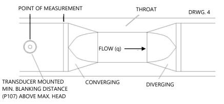
When any **Other** device is chosen please consult the manufacturer of the device for details of where the point of measurement should be located but
