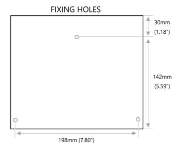
The FlowCERT Lite should be mounted by drilling three holes suitable for size 8 screws (length to suit the application) and fixing the screw in place. Hang the unit on this and fix the two remaining screws by removing the terminal access cover to access the pre-drilled holes.
