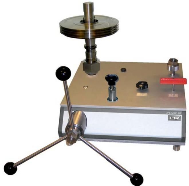
High-pressure Deadweight Tester/Pressure Balance CPB5000-HP
