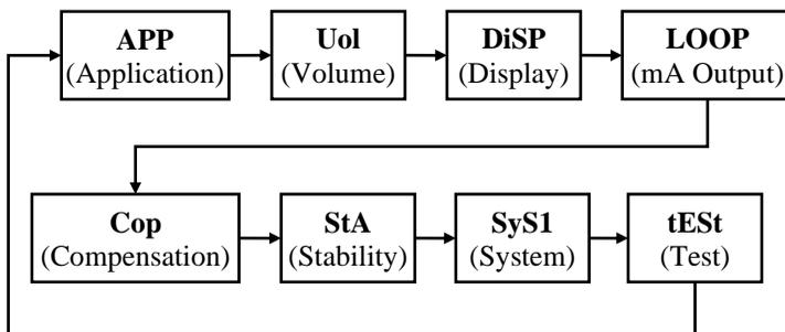
As you press the UP and DOWN buttons to scroll left and right between the menu options, you can press ENTER at any time to select a specific menu which will then take you to the parameters within the selected menu.
