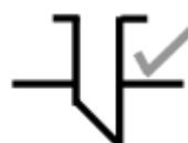
Correct standpipe installation
