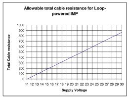
Maximum cable resistance vs supply voltage for 2 wire mode.
