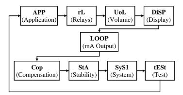
As you press the UP and DOWN buttons to scroll left and right between the menu options, you can press ENTER at any time to select a specific menu which will then take you to the parameters within the selected menu.
