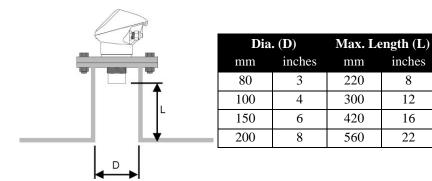
When using a standpipe, fixed to the top of a vessel, ensure that the open end of the standpipe is clear of any obstructions such as weld seams, gaskets etc. in order to avoid unwanted signal returns.
