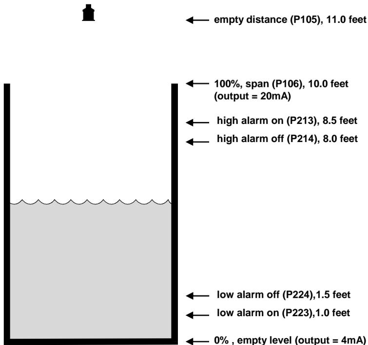
In this example, the blackbox and dB6 is being used to monitor a moving level within a vessel and is required to provide a 4 to 20mA output proportional to the level, over a range of 10.0 feet. In addition, when the level rises to 8.5 feet, Relay '1' is required to give a high alarm and reset when the level falls to 8.0 feet. In the event that the level should fall to 1.0 feet then Relay '2' is to give a low alarm and reset once the level rises to 1.5 feet.
