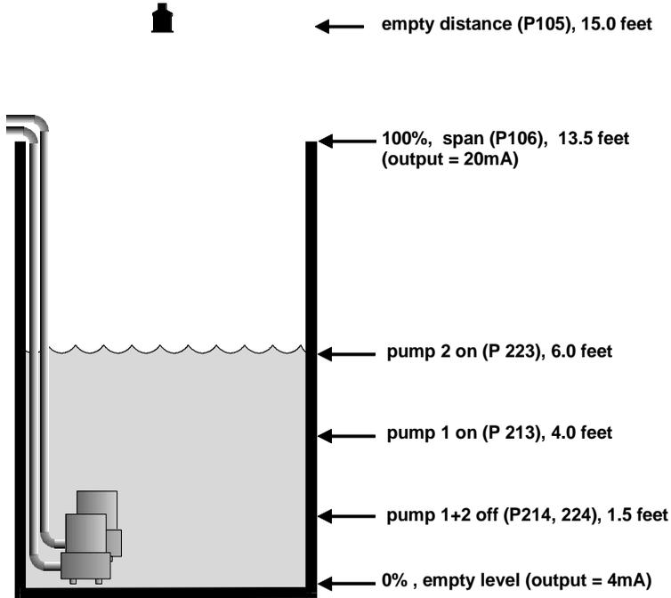
In this example a blackbox with dB6 is being used to control pumps on a **pump down** application, there are two pumps, and the **duty** pump is to be **alternated** between the pumps.
