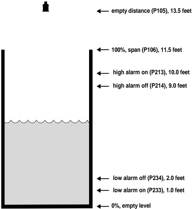
In this example, if the level rises to 10.0 feet, then the high-level alarm (relay 1) will come on until the level drops to 9.0 feet. If the level falls to 1.0 feet, then the low-level alarm (relay 2) will come on until the level rises to 2.0 feet.
