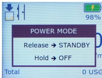
Stand-by mode is intended to be used to put the meter in a low-power state, while keeping the processor awake so that periodic data logs can be made by returning to normal-power, taking the measurement, then returning to low-power standby again. This "standby logging" functionality will form part of a later release, therefore it is not recommended that the meter is placed into standby mode since the battery will drain significantly faster than if completely off.
