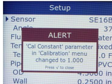
**Angle** – For SE16B only, select angle which matches the transducer pair connected to the PTFM. Options: 35, 37, 39, and 41.
