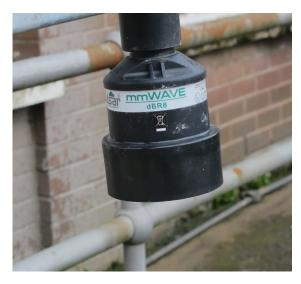
(FFT). The difference between the two, corresponding to the time the signal has taken to return, FMCW is said to be the more accurate because of its narrower beam angle, and in most cases, a stronger signal.
