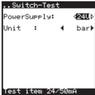
"PowerSupply:" If the unit under test (pressure switch) shall be powered by the LPC 300, set to "24V". Otherwise set to "OFF" to safe battery power.
