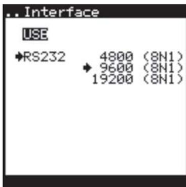
Here you can select the interface for the optional communication with a PC (with the optional software LPC-Cal).
