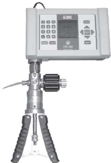
Calibration Setup with Pressure Comparator (spindle pump) as pressure source
