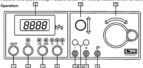
Pressure output P should be connected with 6 mm tube at a low or negative pressure using a T-piece to the pressure to be measured as well as to the pressure intput "+" resp. -" for vacuum. For large displacement volumes the measuring pressure is set to course using the pump [10]. Fine setting is made with knob [11].
