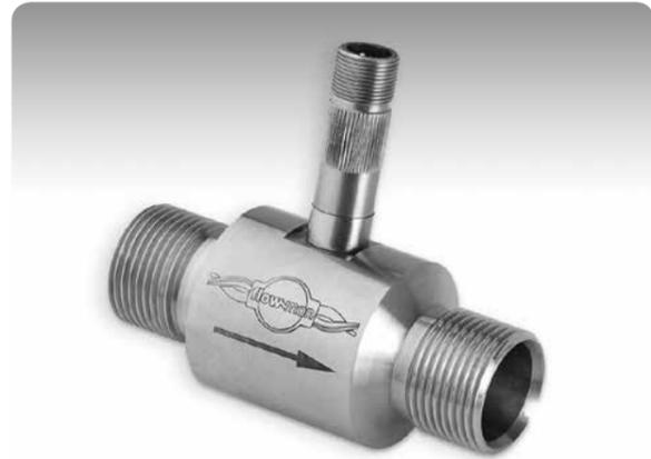
Our Turbine Meters are suited for use on lubricating or non-lubricating liquids of low to medium viscosity and largely insensitive to density variations, pressure or temperature fluctuations. They are available in a wide variety of body sizes and styles, with an electrical pulse output directly proportional to the flow rate.
