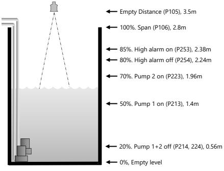
In this example, there are two pumps, which will be set to **alternate duty assist**, so they come on alternately. **Pump 1** is to be set to **Relay 1**, **Pump 2** to **Relay 2**, and the **high-level alarm** to **Relay 5**.
