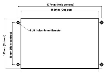
The full dimensions of the fascia mount enclosure are as shown below:
