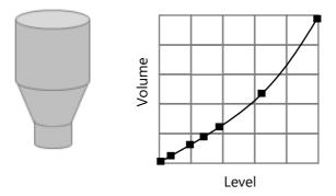
You should enter a level/volume breakpoint for each place where the vessel changes direction, and numerous where the section is slightly curved (mostly linear but has got a small arc). You can enter any number of pairs between 2 and 32.
