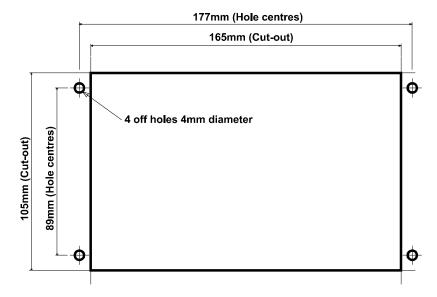
The full dimensions of the fascia mount enclosure are as shown below.
