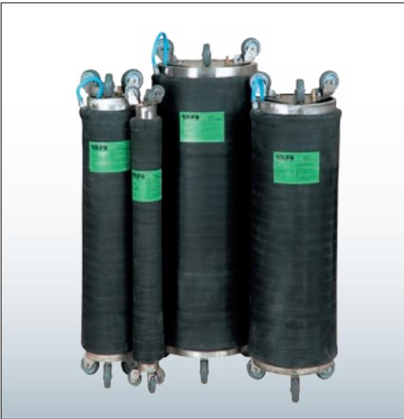
Short packers are provided with an exchangeable two-layer rubberized-fabric sleeve mounted on a metal central part. Moreover, the packers are provided with wheels at both its ends at an angle of 120°. The wheels ensure the stability of the packer in the pipeline. Its design allows water to flow freely during the repair. The length of the effective surface is 600 mm which is sufficient for repairing a joint or a short damaged spot.
