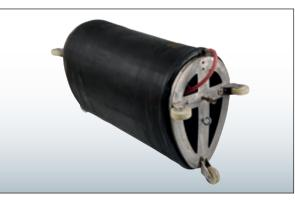
Short packers are provided with an exchangeable two-layer rubberized-fabric sleeve mounted on a metal central part. Moreover, the packers are provided with wheels at both its ends at an angle of 120°. The wheels ensure the stability of the packer in the pipeline. Its design allows water to flow freely during the rapair. The length of the effective surface is 600 mm which is sufficient for repairing a joint or a short damaged spot.
