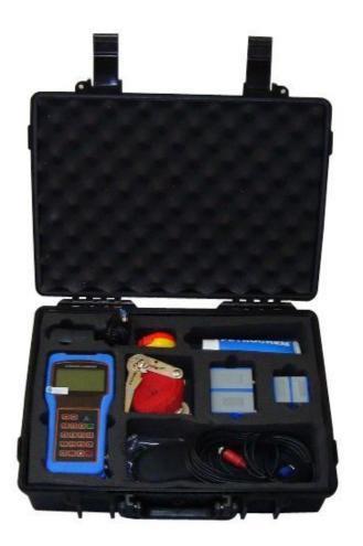
Non-Contacting Flow Measurement Ultrasonic transducers mount on the outside of plastic or metal pipes to measure flow rate of clean, non-aerated fluids like water, chemicals, and oils. The clamp on transducers can be mounted without shutting down flow. There is no pressure drop and no obstruction. Transducer separation distance is calculated by the flowmeter according to pipe diameter and wall thickness.
