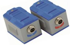
Non-Contacting Flow Measurement Ultrasonic transducers mount on the outside of plastic or metal pipes to measure flow rate of clean, non-aerated fluids like water, chemicals, and oils. The clamp on transducers can be mounted without shutting down flow. There is no pressure drop and no obstruction. Transducer separation distance is calculated by the flowmeter according to pipe diameter and wall thickness.
