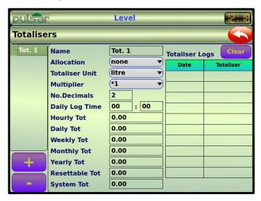
All current **Totaliser Profiles** will be listed by their given names in the tree list on the left-hand side of the screen. Swap between the profiles by selecting a name on the tree list. New profiles can be added by pressing the button or, when selected, delete existing ones by pressing the button.
