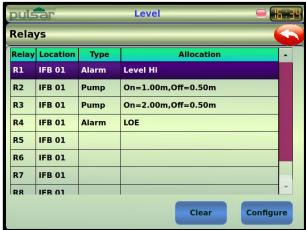
Once you have selected the relay you wish to use and have pressed 'Configure' you will see the screen as detailed on the right. The screen will confirm the Relay number and the Interface Board (IFB) on which it is located, in this case R1 on IFB1\*.
