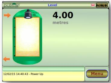
Once the Ultimate has been set up for an application, the display can be configured to show additional information about the application and which features are in use. An example is shown below.
