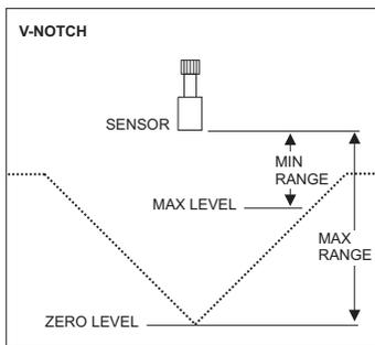
2. Check the maximum range with the sensor installed by:
