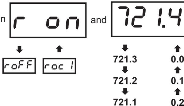
**ROC2** (Level + Echo Loss Alarm) - Relay will be energized when the Relay ON set point is reached.
