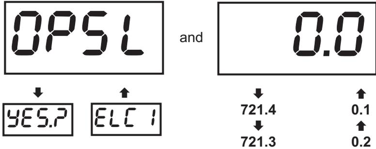
The Output Simulation function controls the digital display 4-20mA output and control relay. Use it to simplify calibration of remote 4-20mA devices such as chart recorders or remote displays, and to test relay set-points.
