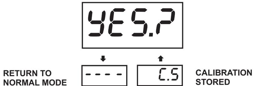
Press **↑** to Store calibration (LIT will display **-C.S-**). Calibration is stored in non-volatile memory (even through power interruptions).
