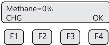
This screen shows the percentage of the gas mixture allocated to methane. In this case, it shows 0%. To program the specific mixture of methane, press **CHG (F1)**.
