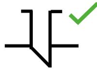
Correct standpipe installation
