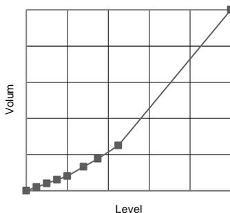
You should enter a level/volume breakpoint for each place where the vessel changes direction, and several where the section is slightly curved (mostly linear but has got a small arc). You can enter any number of pairs between 2 and 32.
